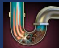
Clogged Drainage System
